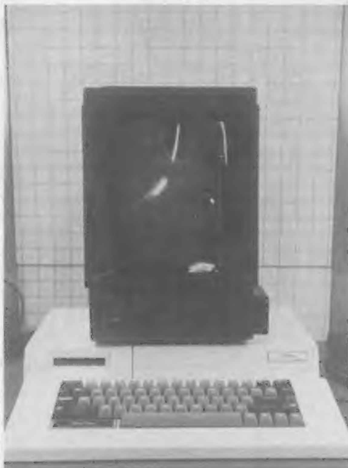
The Vectrex games player sitting on top of the prototype keyboard which turns it into a computer
